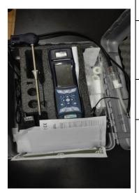
**Device Name:** Industrial Combustion GAS & EMISSION ANALYZER.
